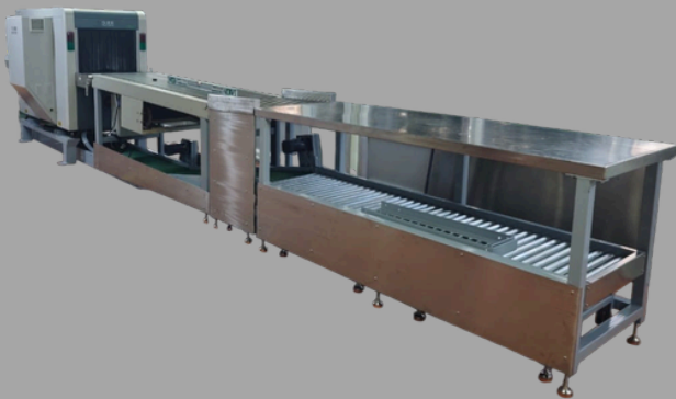
RETURN TRAY CONVEYOR
